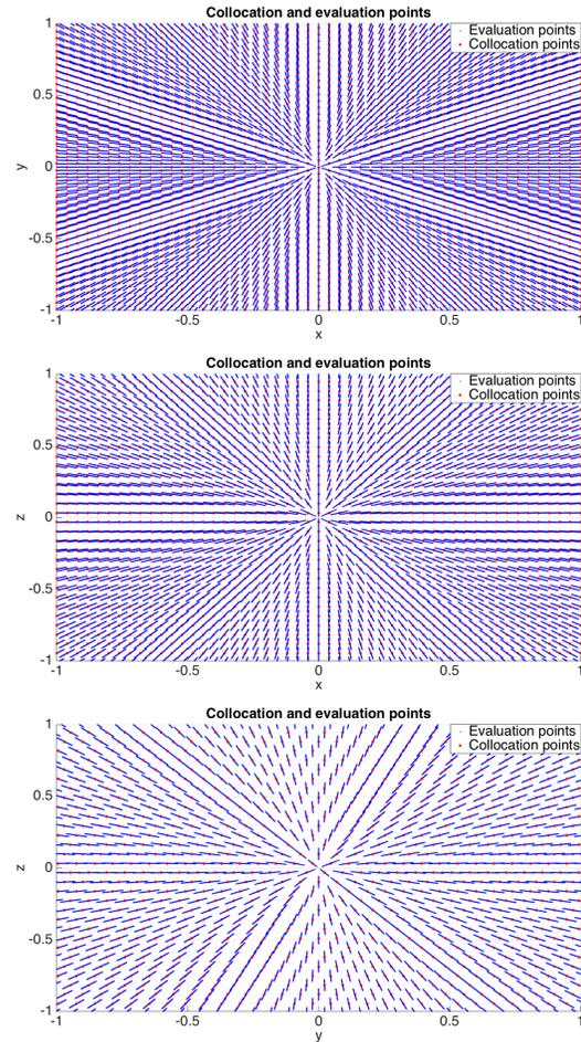
Fig. 1. Collocation and evaluation grids for system (8). First, second and third figures show the XY, XZ and YZ planes, respectively.
