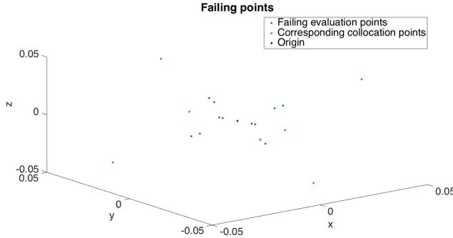
Fig. 3. Chain-recurrent set for system (8). The red points represent the collocation points. The blue points represent the evaluation points to the directional grid. The dark point in the centre of the image shows the origin.
