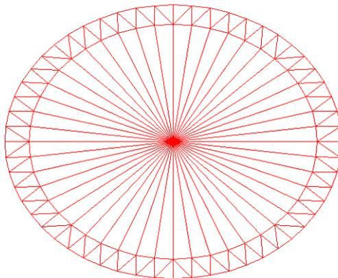
Figure 2: An example of the improved triangulation scheme we propose in two dimensions. Note the triangle-fan at the origin. Additionally, the picture gives an idea of how to extend the triangulation away from the origin. For (3.1) with  $\epsilon = 0.1$  and this triangulation in 48 triangles with the origin as a central vertex, there exists a continuous Lyapunov function that is linear on every triangle in the triangle-fan, cf. Lemma 3.2.
