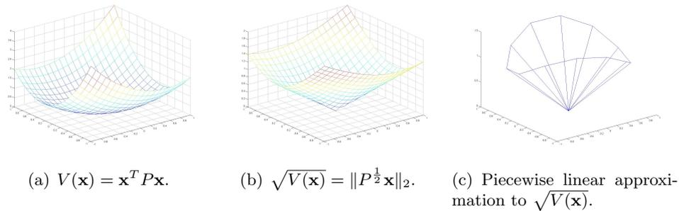
Figure 3: A system with an exponentially stable equilibrium possesses a local quadratic Lyapunov function (a). The square root of this function is also a Lyapunov function (b) and this Lyapunov function can be approximated by a piecewise linear Lyapunov function (c), cf. Theorem 4.3.
